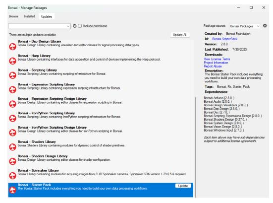
**Note:** Do not enable the "Include Prerelease" option and do not change the "Package Source" to "All" or "nuget.org". Also, do not update the "Bonsai - Harp Library" package. Neurophotometrics.0.6.1 can only use older versions of the harp package.
