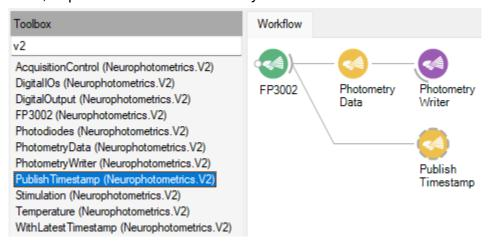
Then, connect the updated "WithLatestTimestamp" node to the data stream to be synchronized with the photometry data, followed by a "CsvWriter" node. In the example below, we synchronize keystroke data using the system's clock with a precision of 1ms.
