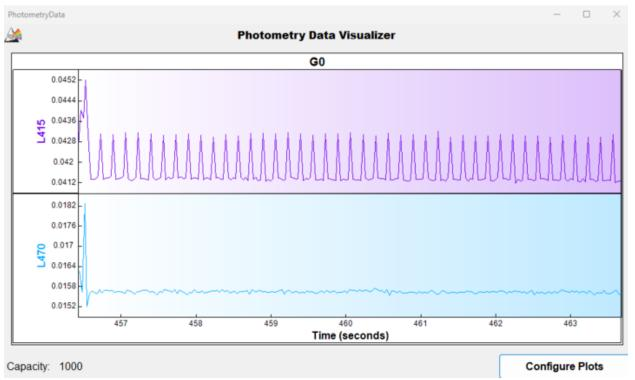
This bug had to do with the AutoCrop feature and so slightly moving an ROI could introduce or fix the issue. Neurophotometrics.0.6.1 has an updated AutoCrop feature that prevents this artifact from occurring.
