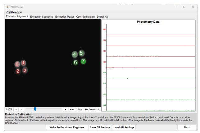
The "FP3002 Setup" window is now segmented into five tabpages helping with different aspects of configuring the FP3002 system: "Emission Alignment", "Excitation Sequence", Excitation Power", "Opto-Stimulation", and "Digital IOs". At the bottom of the window are buttons for navigating the setup window, saving/loading settings, and writing settings to persistent registers on the system.
