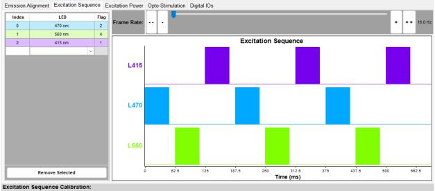
Set the order of the LEDs in a given trigger sequence. Their associated "Frame Flag" values will appear next to the LED names
