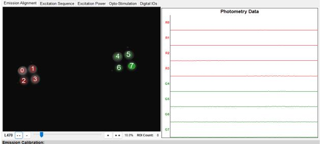
Increase the 470 nm LED to make the patch cord visible in the image. Adjust the 1-Axis Translator on the FP3002 system to focus onto the attached patch cord. Once focused, draw regions of interest onto the fibers in the image that you wish to record from. The image is split such that the left portion of the image is the Green channel while the right portion is the Red channel.
