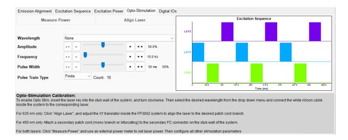
Begin by specifying the "Wavelength" property. If the wavelength is 450nm, then the "Measure Power" button will enable. If the wavelength is 635nm, then both the "Measure
