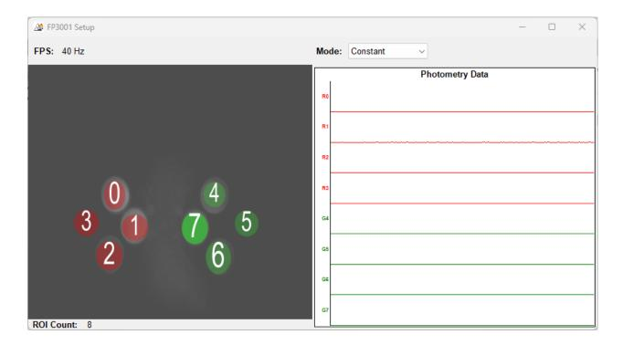
In this window, users can specify the "Mode" property, which replaces the "Trigger Mode" property from previous versions. Also, instead of users calculating the desired "Exposure Time", they instead match the "FPS" property of the "FP3001 Setup" window with the "FPS" specified on the driver box. Below is a description for each property in this updated window:
