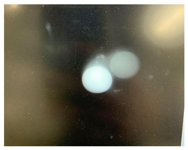
Example of flare that indicates poor alignment.
