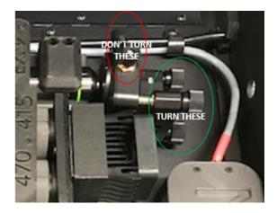
We strongly recommend that you avoid turning the two smaller knobs on the 5-axis translator. These were lined up with the objective lens prior to shipment and very rarely need to be adjusted. They are also *very* sensitive; a little turn can go a long way towards throwing off your alignment!
